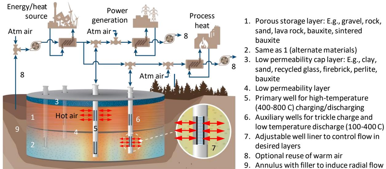
**Figure 1. THERMST™ conceptual design for 10–100 GWh of thermal energy storage [1].**
