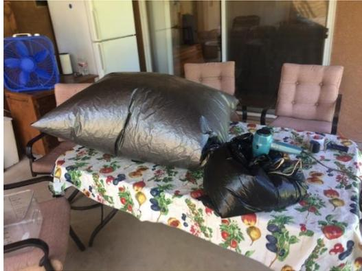
Figure 5. Measurement of airflow using a trash bag.
